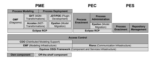
Fig. 2. Overall Architecture of the Integrated Tool Chain
